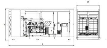
Length, L 4.640 m Heigth, H 1.680 m Width, W 2.4 m Weight, Total 4655 kg
