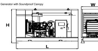
Length, L 2.800 m Heigth, H 1.637 m Width, W 1.100 m Weight, Total 1250 kg
